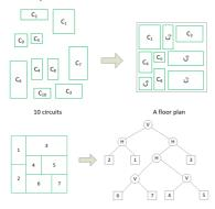
Floor planning problem. Given are *n* circuits of different area requirements. Goal: arrange them into a floor layout so that all circuits are placed in a minimum layout. Each solution candidate can be represented by a tree. Source: Encoding Techniques in Genetic Algorithms, Debasis Samanta, 2018.
