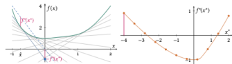
(a) The function f (solid) and the linear function of x^* = -4 (dashed) and its shifted tangent (dotted).
