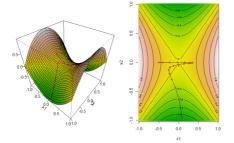
GD was slowing down at the saddle point (vanishing gradient). GD with momentum "breaks out" of the saddle point and moves on.
